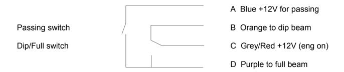
The Grey/Red wire is fed from an engine-on relay, and the Blue is merely ignition controlled.
