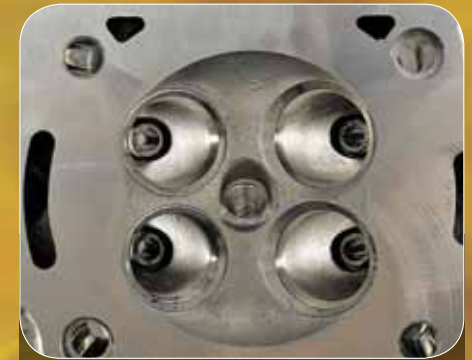
Increase in combustion chamber diameter: from \phi 57 mm to \phi 64 mm
