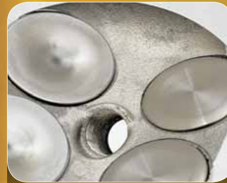
Intake Valve \phi 25 mm - Exhaust Valve \phi 22.2 mm
