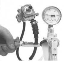
Lack of tightness or the fact that the valve opens at different vacuum values should be regarded as anomalies. In this case, replace it.
