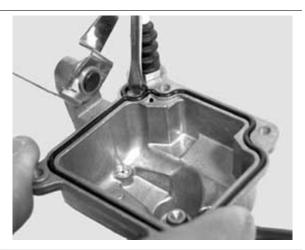
Adequately support the carburettor and using a rod and hammer remove the float pin acting from the throttle control side.
