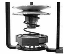
020444Y Tool for fitting/ removing the driven pulley clutch 020444Y011 adapter ring 020444Y009 46x55 Wrench Locking torques (N\*m)
