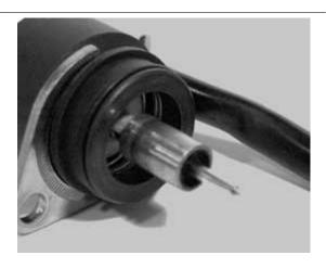
With a 12V battery power the automatic starter and check that the piston protrudes as much as possible.
