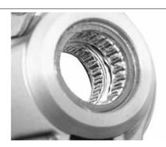
Remove the two roller bearings from the bracket with the specific tool operating on the shock absorber attachment side as shown in the photograph
