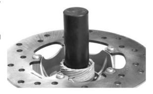
Soap-based lithium grease with NLGI 3; ISO-L-XBCHA3, DIN K3K-20
