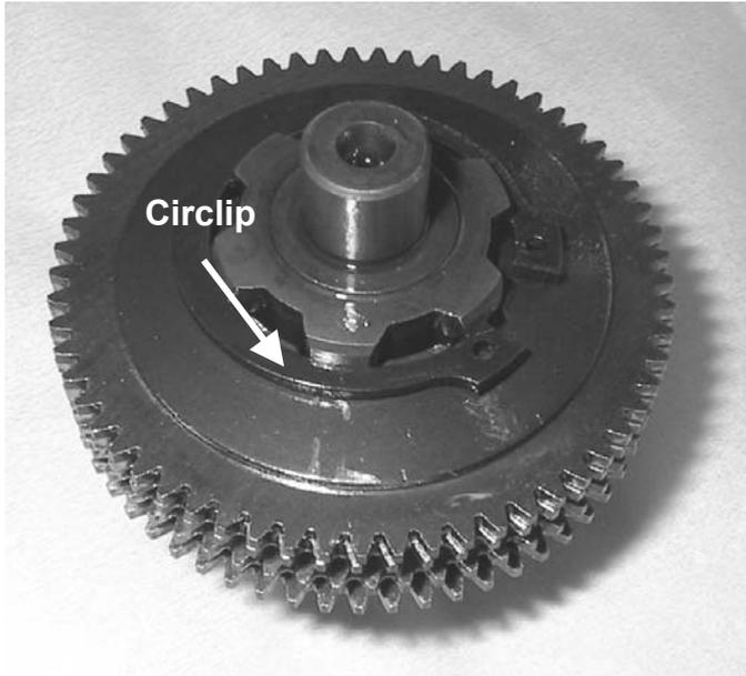
The starter motor intermediate gear is a limited slip gear. The unit is available under a single part number and should **not** be disassembled by removing the circlip.
