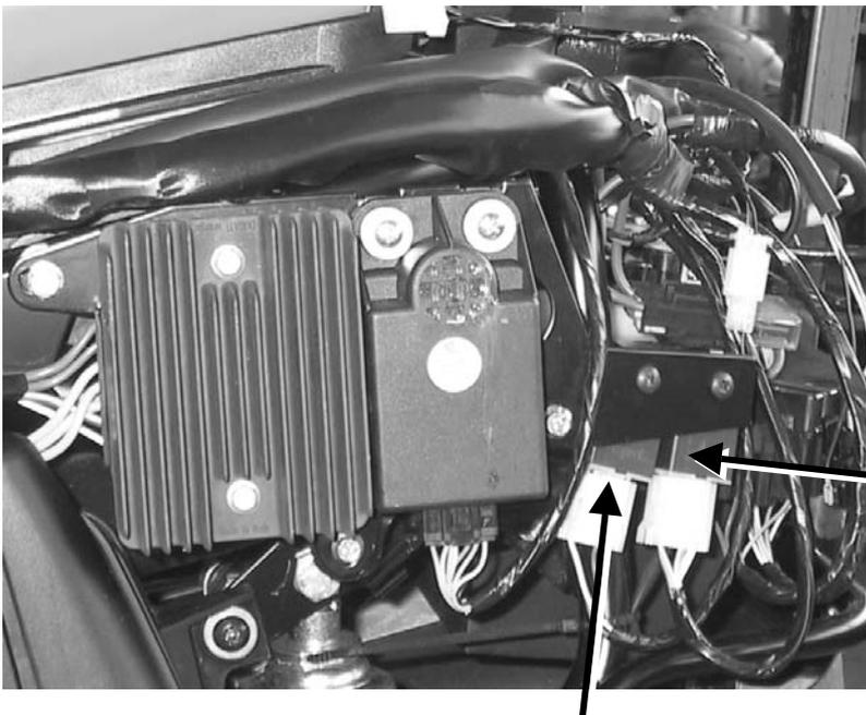
Relay for HT Coil, Fuel Pump and Injector
