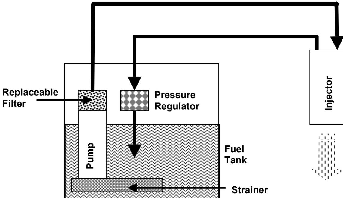
Fuel is drawn through the osmotic strainer by the fuel pump and passed through the filter to the injector. A return line brings fuel back to the tank and the regulator. The pump pressurises to a maximum of **5- 6Bar**, the regulator maintains the pressure to **3Bar**. The EMS CONTROL UNIT always assumes that the pressure in the fuel is at 3 Bar and therefore the opening time of the injector controls mixture accurately.
