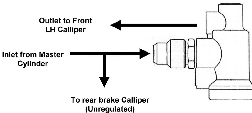
The valve regulates the pressure applied to the front left calliper. The amount of pressure applied is as follows:
