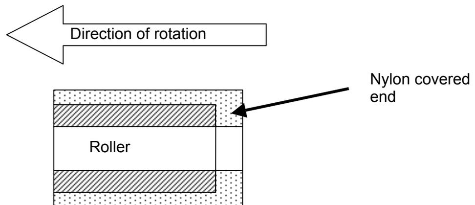
The variator rollers should be fitted dry, this encourages them to roll rather than slide and reduces the flattening wear on the rollers.
