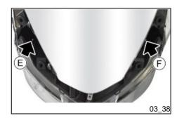
The screw «F» adjusts the height of the left headlight.
