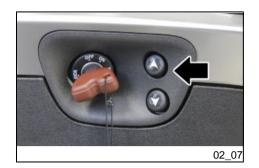
Press on the **«UP»** and **«DOWN»** buttons, after setting the key to **«ON»**, to increase or decrease the rear shock absorber preloading.
