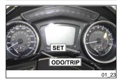
If, during the adjustment procedure, the «SET» button is not pressed for a time longer than ten seconds, the procedure is interrupted and clock value remains the same as before the adjustment; repeat the adjustment operations.
