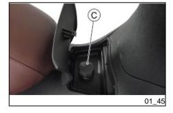
The door automatically rises; to refuel, unscrew the cap «C».
