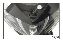
Unscrew and remove the front screw «B».
