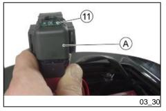
The spare fuse **«11»** is positioned in the same box, but on the side.
