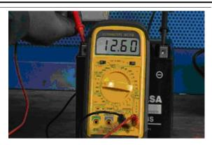
i - The battery is now completely activated, disconnect the battery charger from the fuel supply grid, disconnect the clamps from the battery and proceed to fitting the battery on the vehicle.
