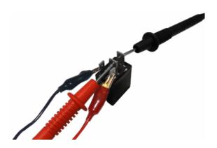
Check the power supply line of the injection load solenoid energising coil: switching to «ON» check the presence of battery tension, for 2 seconds, between the Orange-Blue cable and the Black-Purple cable of the relay base. Otherwise check the continuity of the Orange-Blue cable between the fuse-box and the relay base and of the Black-Purple cable between pin 22 of the control unit and the relay base.
