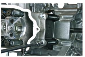
Fit the pins and rocking levers.
