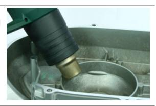
Using the equipment, mount a new bearing, apply grease on the adapter and on the guide in order to maintain the position of the bearing during operation on the vertical axis.
