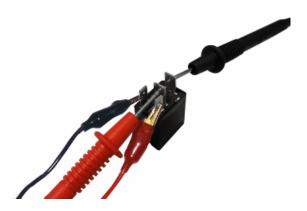
Check the power supply line of the injection load solenoid energising coil: switching to «ON» check the presence of battery tension, for 2 seconds, between the Orange-Blue cable and the Black-Purple cable of the relay base. Otherwise check the continuity of the Orange-Blue cable between the fuse-box and the relay base and of the Black-Purple cable between pin 22 of the control unit and the relay base.
