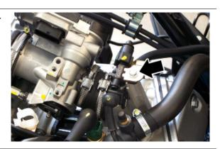
Install the appropriate tool for checking fuel pressure and position the manifold over a container graduated by at least 100 cm<sup>3</sup>. Connect the injector with the cable making up part of the supply for the injection tester. Connect the clamps of the cable to an auxiliary battery. Activate the fuel pump with the active diagnosis. Check that, within fifteen seconds, approximately 40 cm<sup>3</sup> of fuel is dispensed with an adjustment pressure of approximately 2.5 BAR.
