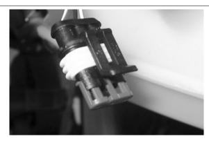
With the ignition switch at «ON» check if there is battery voltage between the Orange-Blue and Black cables.
