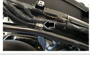
After switching to «ON», check that there is battery voltage, for about 2 seconds, between the Black-Green cable of the pump connector and the ground lead with the pump connector disconnected. Otherwise, check the continuity of the Black-Green cable between the pump connector and the solenoid base.
