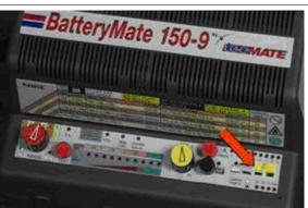
h - Disconnect the clamps from the battery and check the voltage, if voltages are detected of less than 12.8 V, proceed with a new recharge of the battery starting from point c of the recharge procedure of **the new battery**, otherwise go to point i
