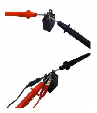
Check the power supply line of the injection load solenoid energising coil: switching to «ON» check the presence of battery tension, for 2 seconds, between the Orange-Blue cable and the Black-Purple cable of the relay base. Otherwise check the continuity of the Orange-Blue cable between the fuse-box and the relay base and of the Black-Purple cable between pin 22 of the control unit and the relay base.
