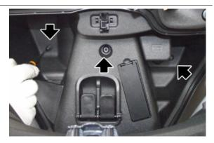
Remove relays and the three connectors from the plate.
