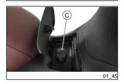
The door automatically rises; to refuel, unscrew the cap «C».
