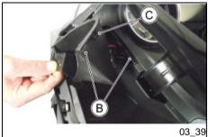
Remove the plastic cover of the glove-box, paying attention to the retainer fins **«B**» (press fit from top to bottom) and **«C**» (lower press fit).
