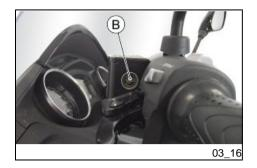
A certain lowering of the level is caused by wear on the brake pads. Should the level appear to be below the minimum mark, please contact an **Authorised Service Centre or Dealer** in order to have a thorough inspection of the braking system carried out.
