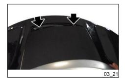
When refitting the components, be very careful not damage the retainer fins of the cover.
