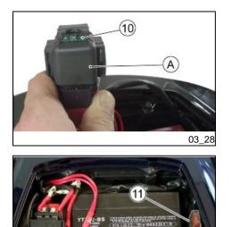
The spare fuse **«10**» is positioned in the same box, but on the side.
