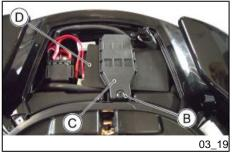
Unscrew and remove the screw  ${}^{\ast}B{}^{\ast}$  and remove the bracket  ${}^{\ast}C{}^{\ast}$  from the rear fitting and the cover  ${}^{\ast}D{}^{\ast}.$
