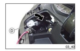
Turn the lamp holder **«D**» by 1/4 a turn clockwise and remove it.
