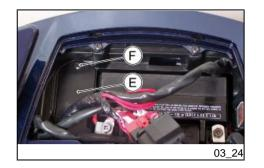
Once the main fuse box  $(A^*)$  is removed, unscrew the screw  $(F^*)$  and remove the cover  $(E^*)$  of the secondary fuse box.
