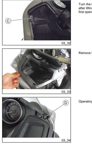
Turn the handlebars to the side opposite to the one on which you are operating and, after lifting the door of the respective dashboard glove-box, unscrew the screw **«C»**, first operating on the left side and then on the right side of the vehicle.
