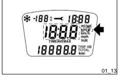
The travel is displayed only if the speed is greater than 5 km/h (3 mph), otherwise the symbol «--.-» is displayed.
