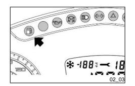
The reserve fuel level is indicated by the warning light on the instrument panel turned on.
