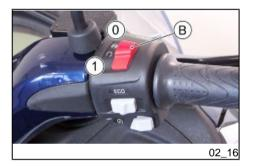
Position the engine stop switch **«B»** to the **«0»** of **OFF** position.
