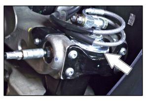
Lock the screw securing the top of the side sleeve to the parallelogram at a torque of 45 ÷ 50 Nm.
