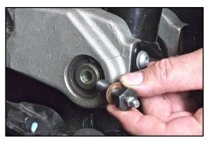
Lock the special tool at a torque of 14 ÷ 20
