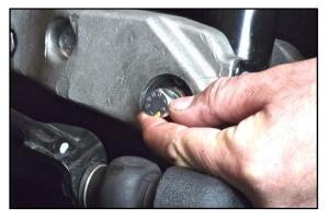
Lock the screw securing the bottom of the side sleeve to the parallelogram at a torque of 45 ÷ 50 Nm;
