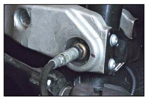
Pump the grease into the housing of the bearing until detecting leakage from the sealing surface of the lower dust gaiter;
