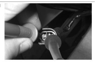
With interface wiring disconnected from the control unit, check the continuity between pin 34 and the brown cable of the tilt locking gripper sensor connector on the system side.
