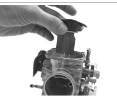
Remove the tapered pin from the vacuum-operated valve
