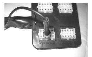
Check the continuity between the black cable on the connector and an earth point on the chassis.
