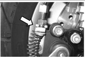
Remove the two fixing screws of the mechanic calliper and remove the calliper. To check calliper components, refer to the chapter on the tilt locking calliper.
