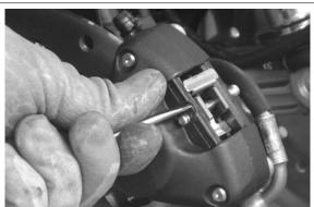
Unscrew the braking splitter screw. Disconnect the brake pipes removing the two metallic straps indicated in the figure. Remove the brake oil tube fitting from the rigid pipe inside the front suspension arm and loosen the hydraulic joint fixing nut of the suspension locking to release the brake pipes.
