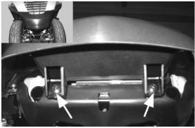
Remove the two rear retainers and then, the two wheelhouse front retainers.
