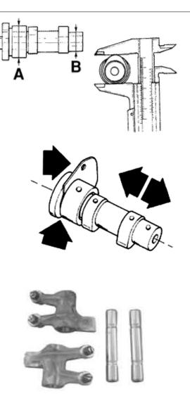
Cam shaft check: Maximum admissible axial clearance 0.42 mm Cam shaft check: Standard axial clearance: 0.11 - 0.41 mm Cam shaft check: Standard height Outlet: 29.209 mm Cam shaft check: Standard height Inlet: 30.285 mm Cam shaft check: Minimum admissible diameter Bearing B diameter: 19.950 mm Cam shaft check: Minimum admissible diameter Bearing A Ø: 36.94 mm Cam shaft check: Standard diameter Bearing B diameter: 19.959 ÷ 19.98 mm Cam shaft check: Standard diameter Bearing A Ø: 36.95 ÷ 36.975 mm
