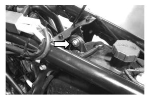
Remove the two lower bracket retainers indicated in the figure.
