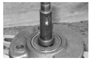
Lubricate the interference areas, match the crankcase halves with slight hits of a mallet to get them into contact.
