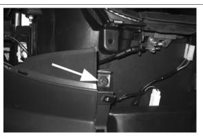
Remove the screw on the fairing front part, pull the fairing to release the hooks. Follow the same procedure for both fairings.
