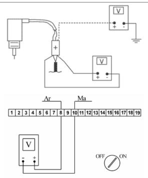
positive probe to terminal No. 8 (Orange), and the negative one to terminal No. 10 (Brown) (see figure).
