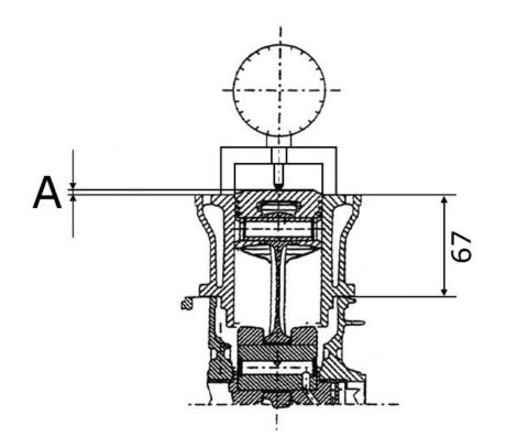
Measurement **«A»** to be taken, is a value of piston protrusion. It indicates by how much the plane formed by the piston crown protrudes from the plane formed by the upper part of the cylinder. The further the piston protrudes from the cylinder, the thicker the base gasket to be used (to restore the compression ratio) and vice versa.
