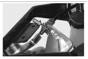
Remove the electrical connection of the geared motor position potentiometer.
