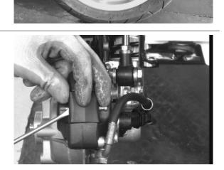
Remove the pad pin lock with a screwdriver, paying attention not to spoil the calliper surface treatment.
