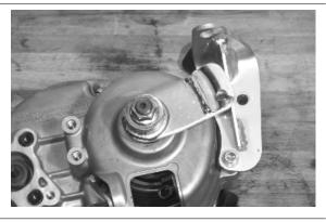
Remove the two bracket screws after releasing the spring and freeing the flexible transmission adjustment.
