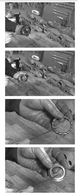
Check the ball bearings on the parallelogram arms. Replace them in case of signs of abnormal wear.
