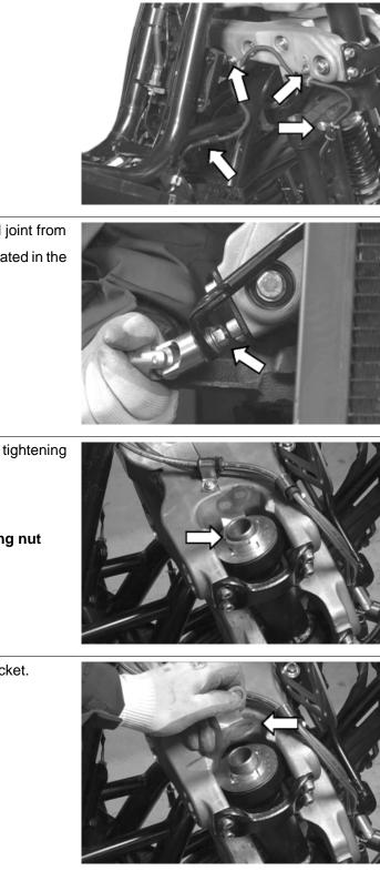
Remove the constant-velocity universal joint from the steering bar by undoing the nut indicated in the photograph.
