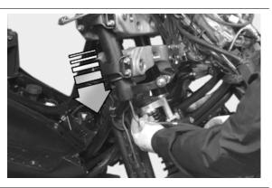
Remove first the flexible part of the calliper from the steering tube as shown in the photograph, and then remove the rigid part.
