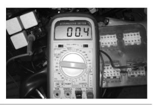
Check the continuity of the yellow - red cable between the pressure switch connector and the fusebox and between the remote control base and the fuse-box.
