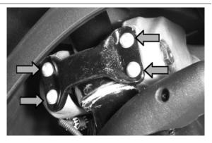
• Remove the right upper screw and the left bottom screw of the parallelogram unit .
