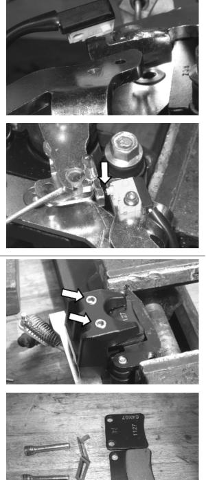
Unscrew the two pad pin screws, remove the pads with the spring.
