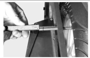
• Check that the pointers of both tyres are correctly aligned, as shown in the photograph. Maximum misalignment allowed: 4 notches
