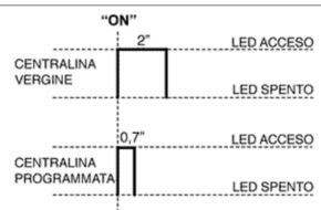
When the key switch is turned to "ON", this blinking function is deactivated. A flash then confirms the system has switched to "ON".
