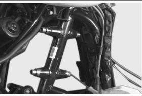
For refitting, follow the operations for removal but in reverse order, lubricating the locking pins on the parallelogram half-arms and observing the prescribed torques.
