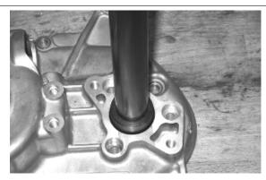
Hold the crankcase in a perfectly horizontal position, heat it with a heat gun at a temperature of about 120 °C, use the specific tool to fit the bearing of the flexible transmission lever control shaft. Hit slightly with a mallet if necessary. Refit the bearing check seeger ring.
