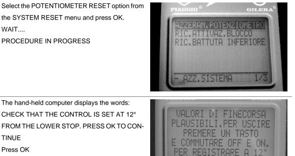
The hand-held computer displays the words: POS-SIBLE LIMIT STOP VALUES. PRESS A KEY AND SHIFT OFF AND ON
