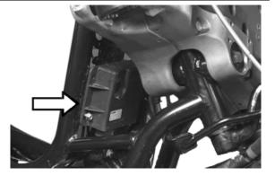
Remove the arm coupling retainers from the parallelogram by loosening the retainers indicated. For easy refitting operations, remember to take note of the positions of the components.
