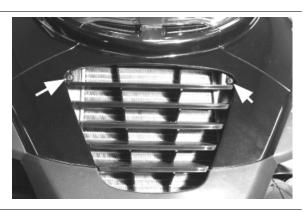
Remove the two lower retainers with the bushing
