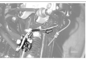
Disconnect the tone wheel connector indicated in the photograph.
