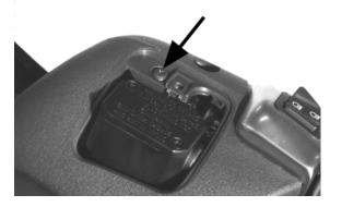
Unscrew the two pairs of screws in the lower part of the half-handlebar.
