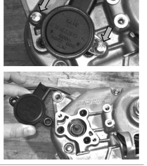
Remove the nut indicated in the figure, if necessary lock the lever with a vice making sure not to spoil the surface.
