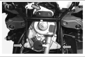
Use a screwdriver to remove the plastic access cover to the pump joint/geared motor
