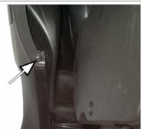
Remove the five screws on the right side and the five on the left side, indicated in the figure.
