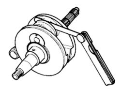
Check the radial clearance on the connecting rod.
