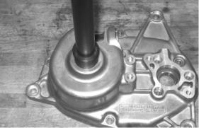
Extract the electric motor bearing with the specific tool.
