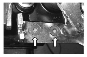
Unscrew the Allen screw and remove the switch. When refitting, place the switch with the button oriented to the stop indicated on the calliper lever; observing the reference indicated on the switch supporting bracket.
