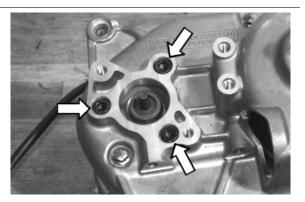
Remove the four screws indicated in the figure, remove the flexible transmission supporting bracket, separate the two crankcase halves, if necessary, use a rubber mallet to hit the flexible transmission lever in order to separate the two crankcases.
