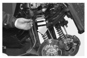
Remove the tone wheel wiring by disconnecting the connector on the fuel tank after removing the chassis central cover.
