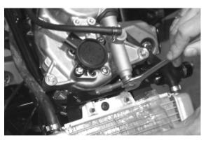
Remove the 3 fixing screws indicated and remove the whole geared motor.
