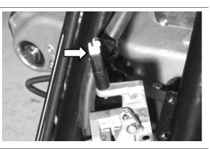
Remove the parking brake cable from the lever by operating the set screw indicated in the photograph.
