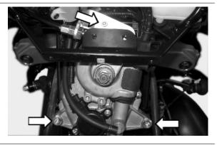
Remove the hydraulic pipe retainers from the parallelogram.
