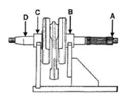
To install the drive shaft on the support and to measure the misalignment in the 4 points indicated in figure.
