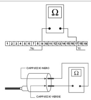
Disconnect the spark plug cap from the HV cable and measure the resistance between the HV cable terminal and the HV coil negative terminal (see figure). If non-conforming values are measured, replace the HV coil. To carry out a more complete diagnosis, check the peak voltage with the multimeter adaptor.
