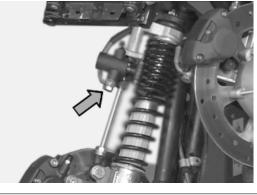
Remove the suspension tilt locking device pipes from the headstock.
