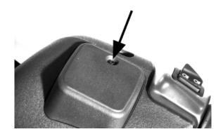
Remove the two screws under the brake pump caps previously removed.
