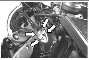
Remove the retainers indicated in photograph of the half-arms joint flange.
