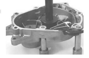
WHEN FITTING THE BEARINGS ON THE ENGINE CRANKCASE, SUPPORT THE CRANKCASE PREFERABLY ON A SURFACE TO ALLOW THE BEARINGS TO BE DRIVEN VERTICALLY.
