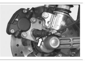
Remove the hydraulic pipe fitting from the sliding locking device, making sure again that the liquid drained is collected.
