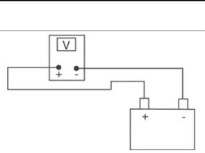
In case of voltage values lower than 14 Volt, check
