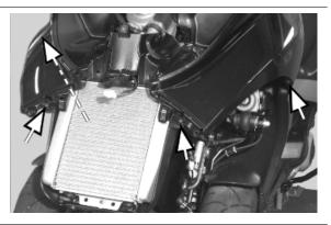
Remove the four screws on the shield back plate.
