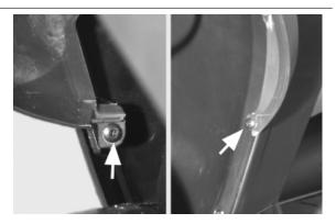
To remove the shield central finishing, remove the PIAGGIO clip-on badge paying attention not to spoil the paint, unscrew the screw underneath and remove the finish carefully.
