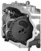
Assemble the limiting bell using the counterweight fixing screw as a reference.
