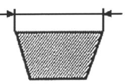
During the wear checks foreseen in the scheduled maintenance services at 6,000 km; 18,000 km; etc., check that the rim bottom of the toothing does not show signs of incisions or cracking (see figure): The rim bottom of the tooth must not have incisions or cracking; if it does, change the belt.
