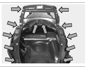
Remove the rear case internal screws indicated in the photograph, to detach the supporting plates of the voltage regulator on one side and the saddle opening switch on the other.
