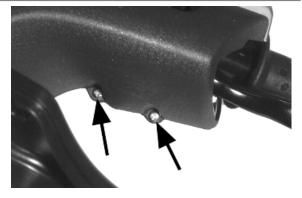
After removing the front part of the handlebar cover, access the two screws fixing the rear part to the handlebar, as indicated in the photograph.
