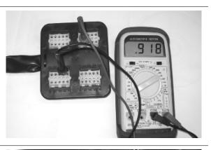
With interface wiring disconnected from the control unit, check the continuity between pin 23 and the brown cable of the LEFT wheel revolution sensor connector; between pin 17 and the red cables of the LEFT wheel revolution sensor and brown cable of the RIGHT sensor; between pin 24 and the red cable of the RIGHT wheel revolution sensor
