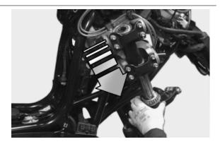
Check that the roller tapered bearing does not show signs of abnormal wear. If it is, replace it.
