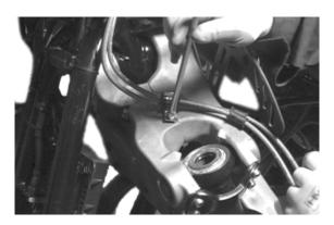
Remove the 4 screws fixing the tilt brake disc sector indicated in the photograph.
