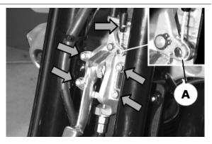
Remove the electric connection from the engaged parking brake warning light switch.
