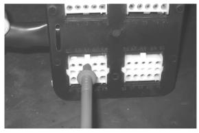
In case of failures, check the continuity between pin 23 and the connector green cable on the fuel tank after removing the chassis central cover; between pin 17 and the yellow cables on both connectors; between pin 24 and the red cable on the connector.
