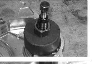
Refit the spring/toothed sector unit, hold the crankcase in a perfectly horizontal and stable position, place the spring/toothed sector unit keeping it perfectly perpendicular to the bearing already fitted on the crankcase; if necessary, slightly hit the unit shaft end with a mallet and protect the thread by screwing in a nut.
