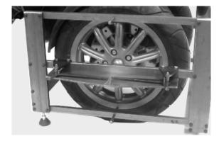
Make sure the frame is adequately centred by checking with a gauge that the lugs along the vertical axis show the standard protrusion.
