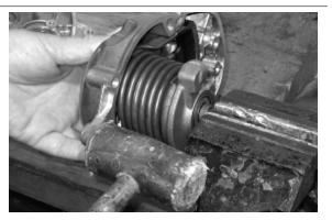
Extract the bearing of the spring/toothed sector unit with the specific tool.
