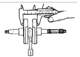
If the axial clearance between crankshaft and crankcase exceeds the standard and the crankshaft does not have any defect, the problem must be due to either excessive wear or wrong machining on the engine crankcase. Check the diameters of both bearings of the crankshaft according to the axes and surfaces shown in the figure. The half-shafts are classified in two categories Cat. 1 and Cat. 2 as shown the chart below.
