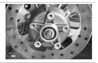
Undo the wheel hub nut. - When refitting, secure to the specified torque.
