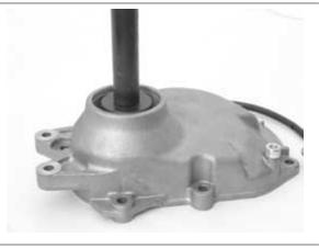
With the appropriate tools, remove the oil seal as shown in the figure.
