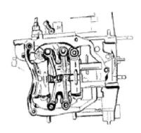
Fit the pins and rocking levers.
