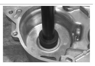
Hold the crankcase in a perfectly horizontal position, heat it with a heat gun at a temperature of about 120 °C, use the specific tool to fit the bearing of the electric motor. Hit slightly with a mallet if necessary.
