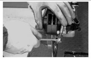
Loosen the two screws indicated in the figure and remove the calliper from the support.
