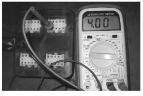
With the interface wiring disconnected from the control unit, check the continuity between pin 17 and the yellow cable of the potentiometer connector, between pin 25 and the green-blue cable, between pin 11 and the orange-blue cable. Also check that these lines are insulated from each other and earth.
