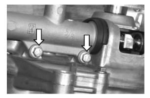
Unscrew the two potentiometer screws. When refitting, plug the potentiometer in D-type connector, afterwards place it with its electric connection directed to the opposite side of the pump.
