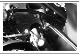
• Fit the steering guiding bracket in a straight riding position, fix one end to the attachment of the half-arm coupling flange and the other end to the screw fixing the steering control arm.
