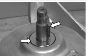
Refit the electric motor; check the position is correct by means of the reference indicated during removal.
