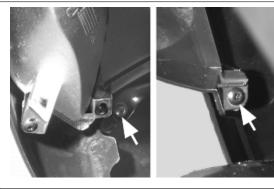
Remove the two screws fixing the radiator lower protection to the shield back plate.
