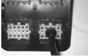
With the interface wiring disconnected from the control unit, check the continuity of the geared motor winding placing the multimeter probes on pins 28 and 38 as indicated in the figure
