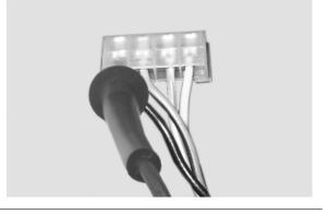
With a multimeter, check the operation of the tilt locking-unlocking switch referring to the diagram indicated in the figure.
