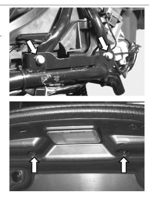
Remove the upper frame, unscrewing the ten upper screws, the two saddle closing screws and the case light wiring.
