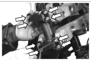
To facilitate the operations indicated below, remove the suspension locking electronic control unit indicated in the photograph.
