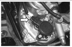
Remove the electrical connection of the geared motor electric motor.
