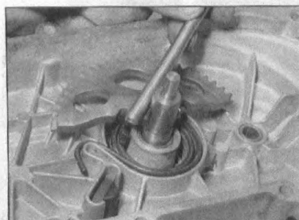
2.11c . . . then locate the steel rod onto the spring end and against the pinion . . .
