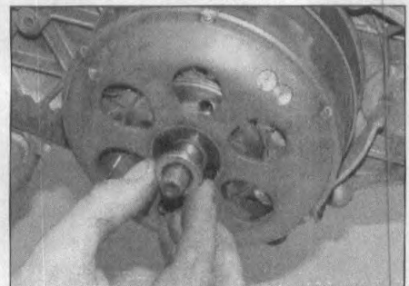
2.6b Note the spacer on the gearbox shaft
