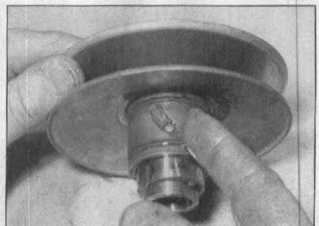
4.9b Apply grease to the slots and around the O-rings
