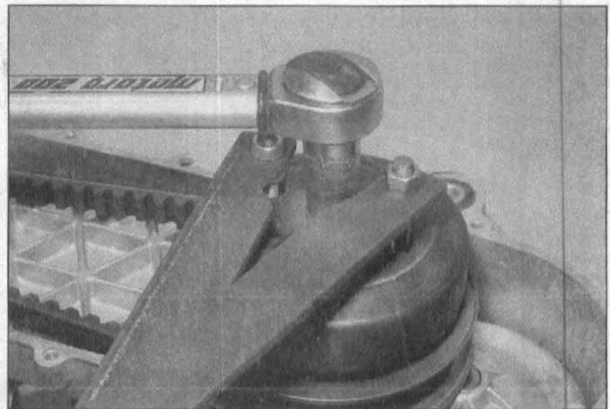
4.12b . . . and tighten it to the specified torque
